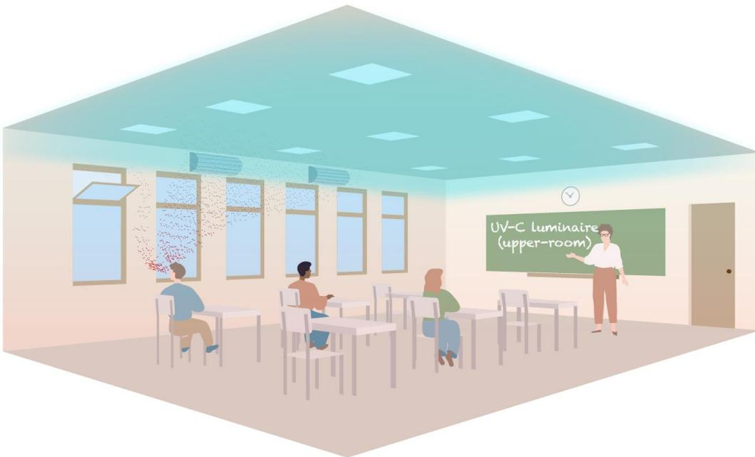
Figure 4: Illustrative example of UVGI upper-room luminaire application
