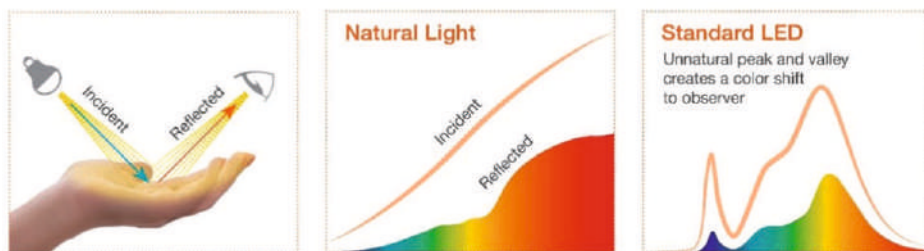
Fig : Effect of Incident Spectrum on Color Rendering
