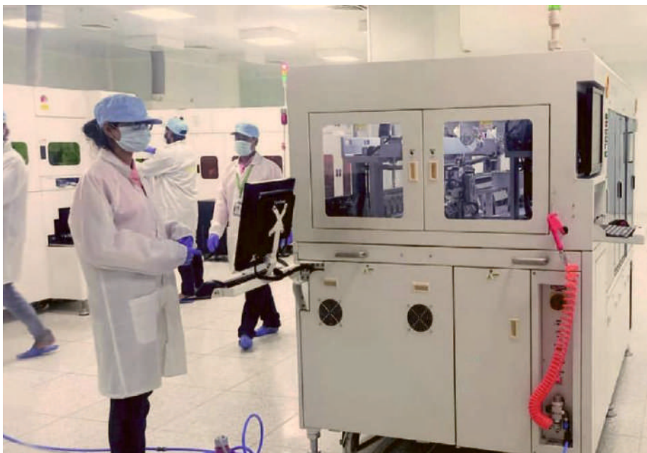
The chip assembly plant at Sahasra's factory in Bhiwadi is capable of packaging 6-12 inch wafer
