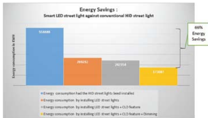
Fig 2.69% Power Savings against conventional HID Street Light Energy savings due to different features of LED Street Light enabled with SMART Control System Owlet
